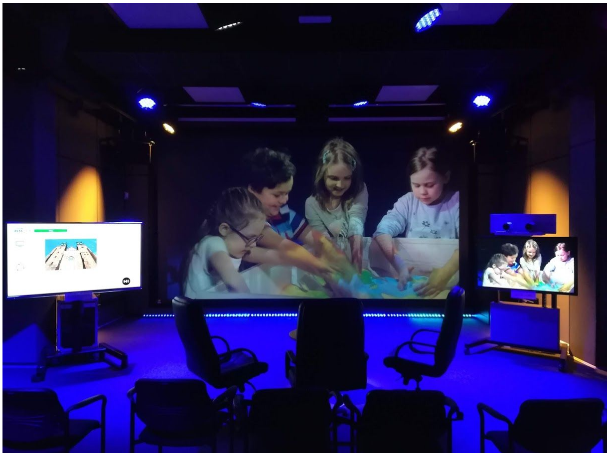
Figure 29: Internal demo for employees and invited guests. PSNC 8K 3D video wall working with the new player. Main screen with 8K content (center), auxiliary content (left-side) and 360 video (right-side) - all of them synchronized
